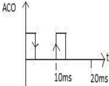
Figure 5 : Analog comparator output of microcontroller
