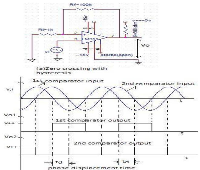
Figure 4 : Comparator and its input, output wave shape
