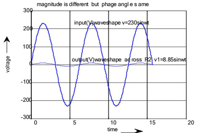
Figure 3 : Input (AC, 230v) and output (V) across R2
