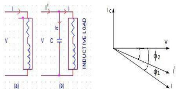
**Figure 1 :** Power factor improvement circuit and phasor diagram
